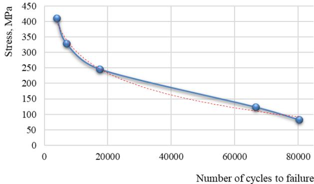
Figure 3 Weller's curve stress-number of cycles S-N
