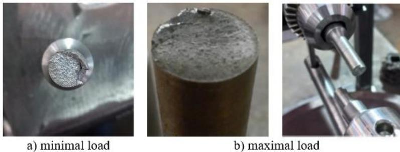
Figure 4 Fracture of the specimen under different loads
