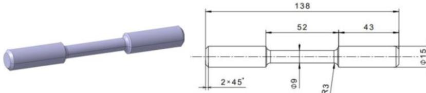
Figure 2 Test specimen made of material C10
